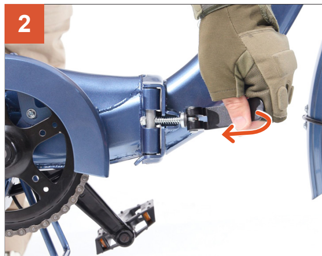
2 Turn the quick release handle clockwise.
