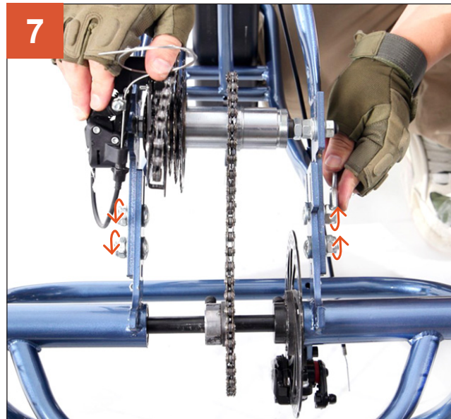
Tighten all 4 sets of bolts and nuts on both frames completely.
