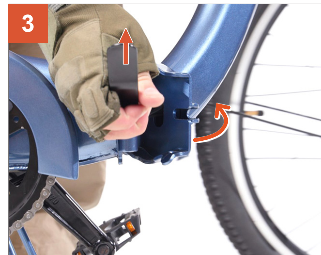
3 Lift the handle with one hand and fold the tricycle with the other hand.
