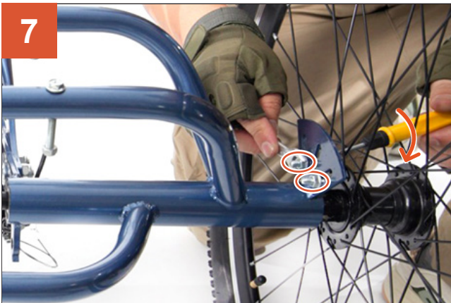
7 Remove the preinstalled bolts, nuts, and washers on the rear frame.
