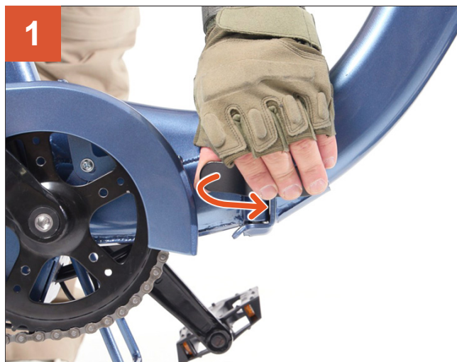
1 Unlock the folding quick release.
