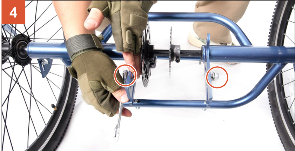
4 Loosen the 2 sets of bolts and nuts on the rear frame with the 17 mm wrench. (DO NOT remove the bolts and nuts.)
