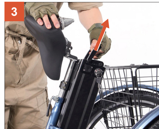
3 Hold the handle at the top of the battery, lifting the battery away from the tricycle.
