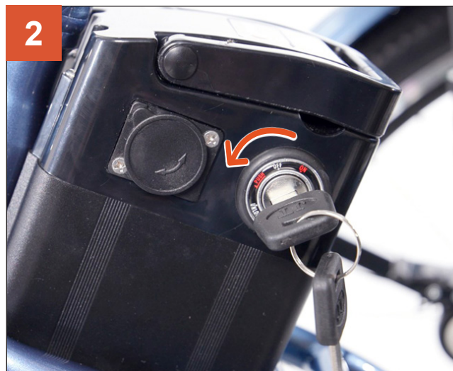
2 Insert the key, turning it counterclockwise to UNLOCK .
