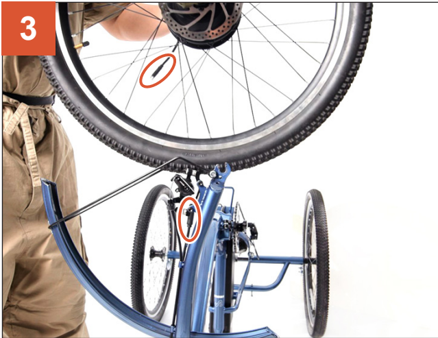
3 Keep the motor cable on the right.
