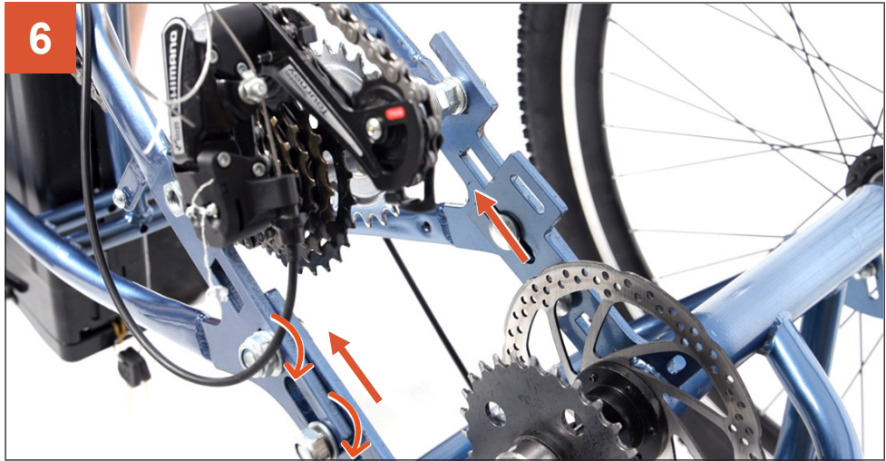
6 Replace the removed 2 sets of bolts and nuts and partly tighten all 4 sets of bolts and nuts on both frames. (Fully tighten them later after rear chain installation.)
