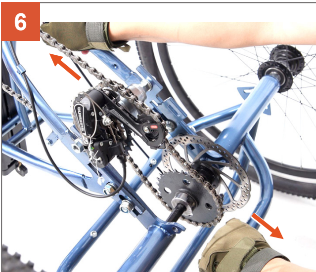
Push the main frame forward until the rear chain is taut.
