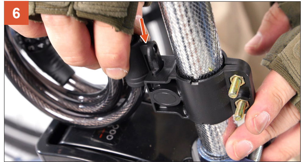
6 Insert the cable lock into the lock bracket.
