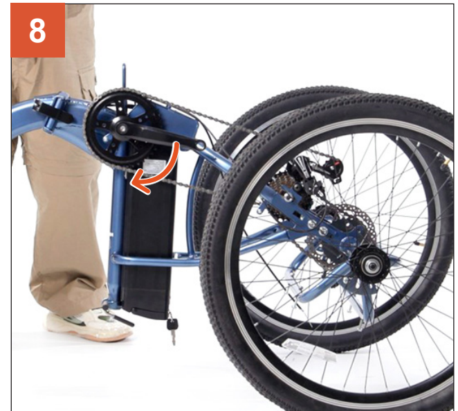
Test that the chains move freely by rotating the right crank arm.
