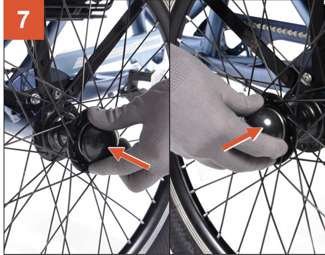
7 Attach the rear wheel caps to the rear wheel hubs, pressing hard until they are locked in place.
