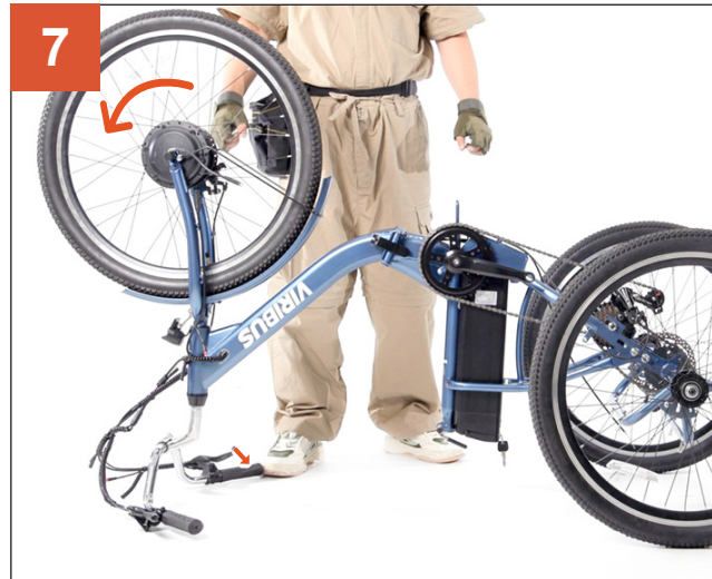
7 Turn the front wheel and press the front brake lever to test the wheel and the front brake.
