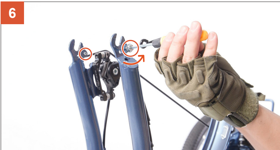
6 Loosen and remove the two preinstalled bolts on the front fork tips.
