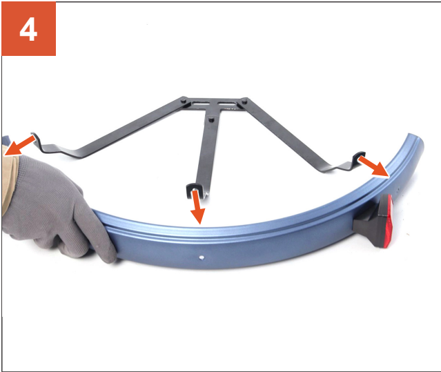
4 Align the rear fender stay with the rear fender.
