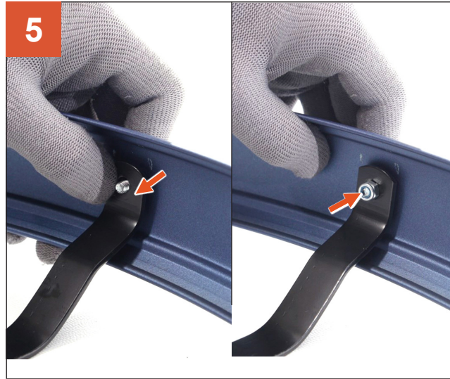
5 Replace the removed bolts and nuts.
