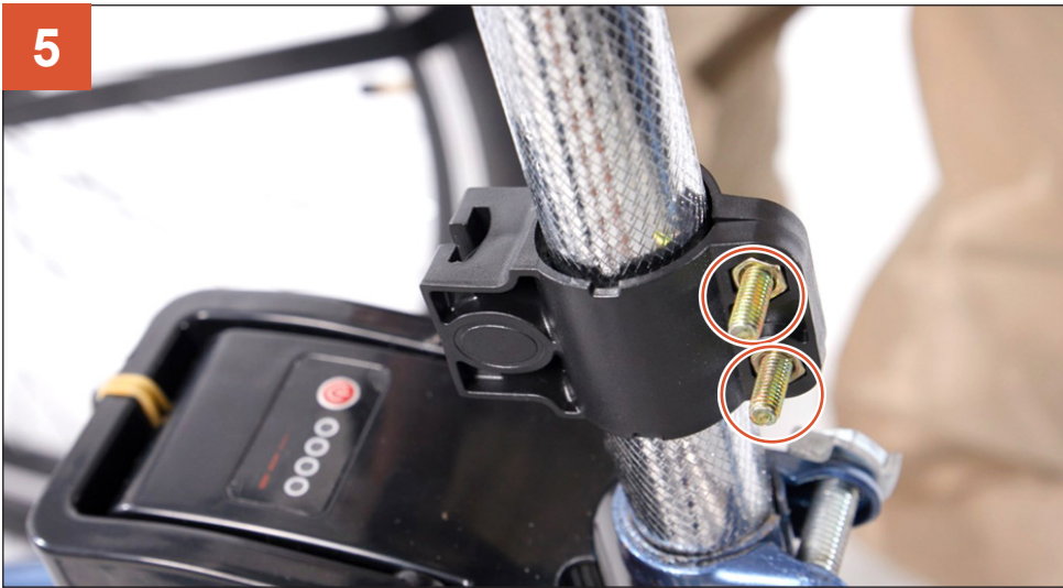
5 Place the lock bracket onto the saddle post using its clamp, and replace and tighten the removed bolts.
