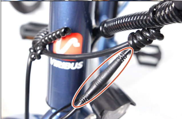
Connect the wiring from the handlebars to the front light.
