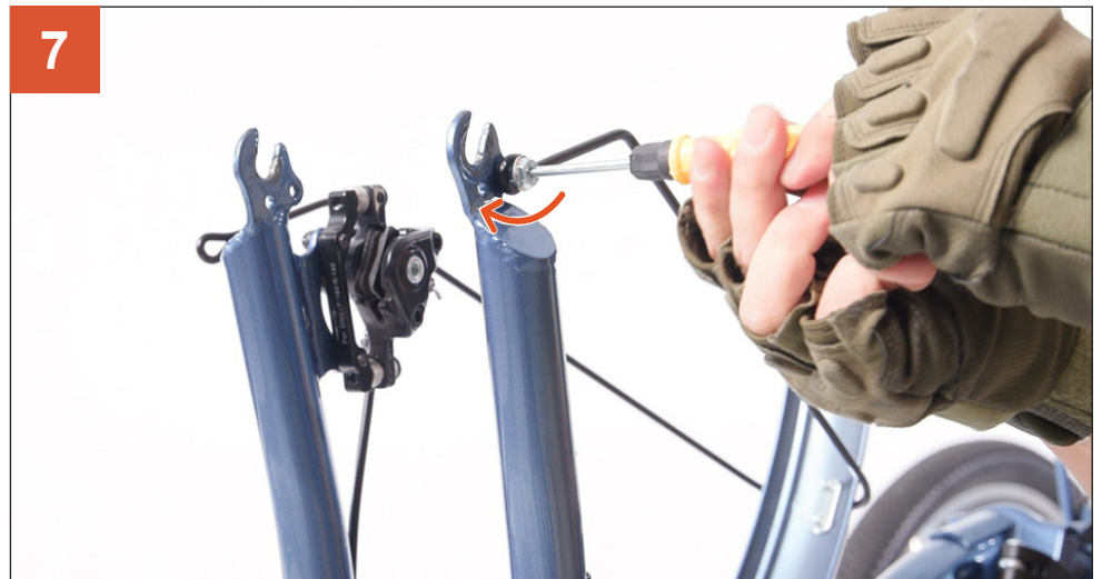
7 Install the front fender stay using the removed bolts.
