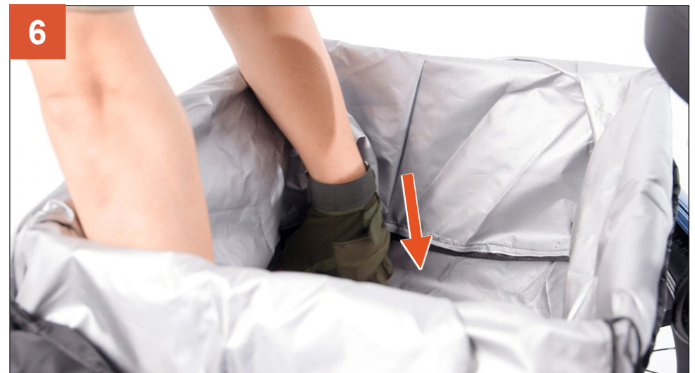
6 Unfold the basket bag and fit it into the basket.
