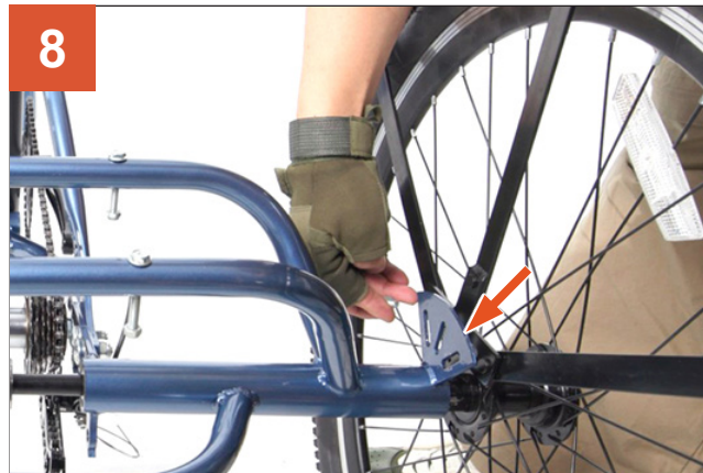
8 Align the fender stay and the rear frame.
