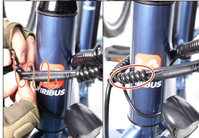
Arrange the wiring with the wire loom tubing.
