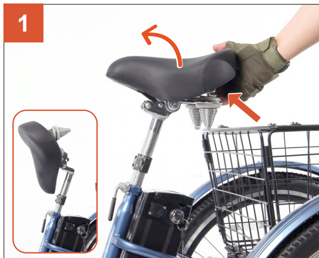
1 Push up the locking lever, raising the rear of the saddle as shown.
