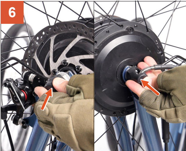
6 Replace the caps, pressing hard until they are locked in place.
