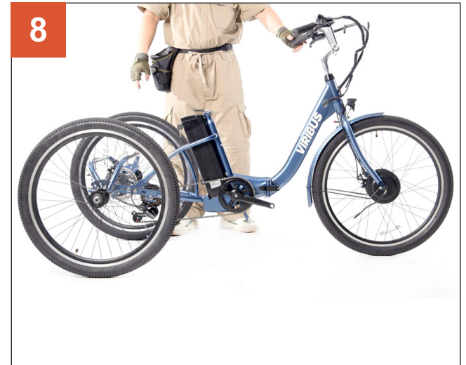
8 If the front wheel is spinning smoothly and the front brake is functioning, turn the tricycle right side up.
