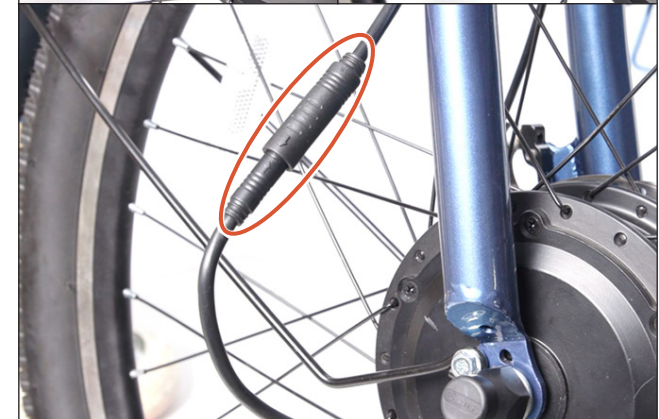
Connect the wiring from the handlebars to the motor.
