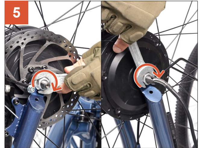
5 Retighten the nuts on both sides.
