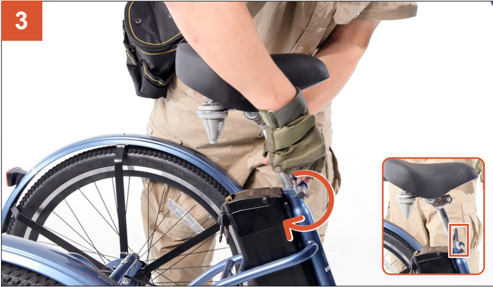
3 Retighten the locking bolt to secure the saddle.
