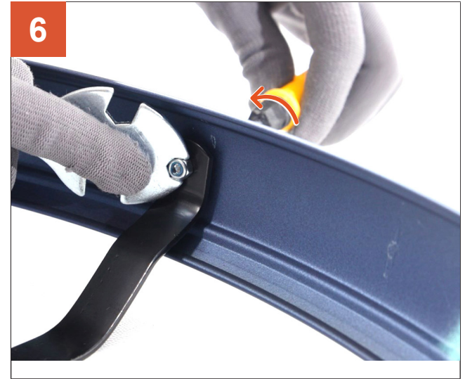
6 Tighten the bolts.
