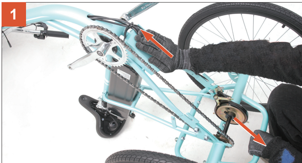
1 Push the main frame forward until the chain is taut.
