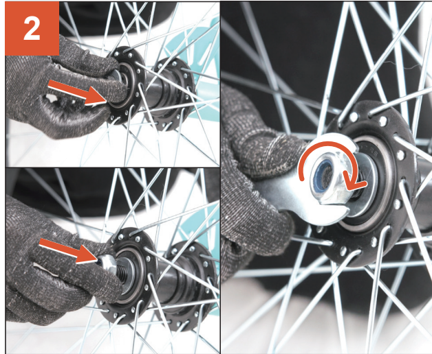
2 Replace the washer and nut, tightening the nut with the 22 mm wrench.
