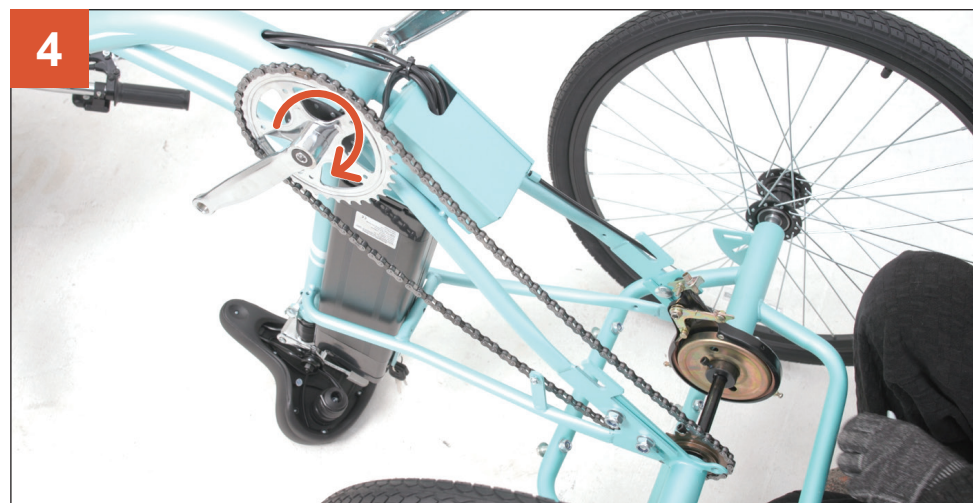
4 Test that the chain moves freely by rotating the right crank arm.
