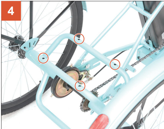
4 Remove the 4 sets of nuts, washers, and bolts from the rear frame.
