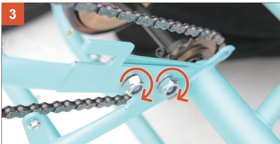
3 Tighten the nuts and bolts completely.
