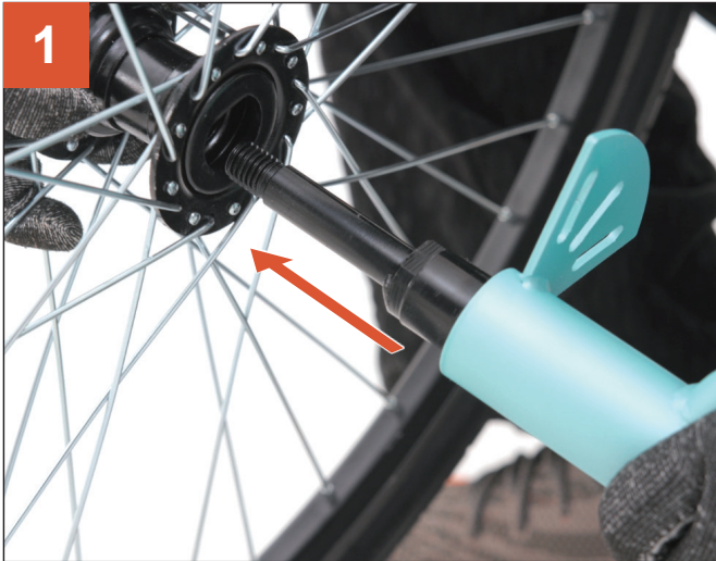
1 Connect the wheel with the D-shaped slot to the hub.
