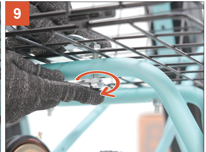
9 Tighten the nuts with the multifunctional wrench and the 22 mm wrench.
