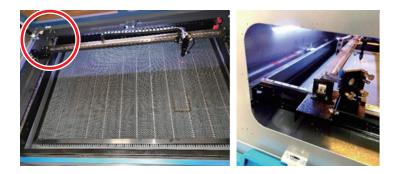
Once set, place a piece of tape on the 2nd mirror's frame. **DO NOT** place the tape directly onto the mirror. Repeat the steps from §5.4.1. If the laser is not centred on the 2nd mirror, you will need to adjust the 1st mirror's set screws accordingly.
