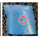
When the laser is well centred along the entire path from the tube to the workbed, your laser mirrors are all correctly calibrated and (assuming they are clean) performing at optimum efficiency.
