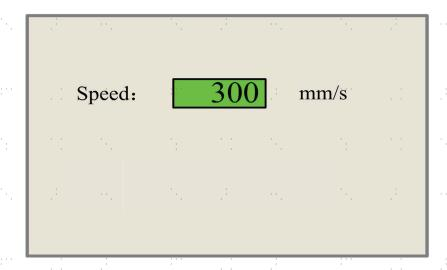
A cursor will appear when pushing  $\bullet$  or  $\triangleright$ . Move the cursor to the numeral area and push  $\blacktriangle$  or  $\blacktriangledown$  to change the value. Press **ENTER** to save the change. Press **ESC** to invalidate the change and return to the main interface.
