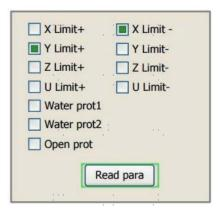
This interface contains input/output information of the system's hardware. Press Read Para. to access hardware information. When the hardware signal is triggered, the small box to the left of the corresponding item will be displayed in green, otherwise it will be grey. Press ESC to return to the previous menu.
