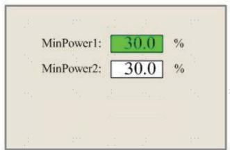
When  $\mathbb{Z}/\mathbb{U}$  is pushed, the green block can move up and down to denote the changing item. Then  $\triangle$  or  $\nabla$  and  $\leftarrow$  or  $\Rightarrow$  can be used to change the value. Press **ENTER** to save the change. Press **ESC** to invalidate the change and return to the main interface.
