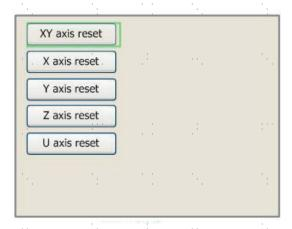
Push ▲ or ▼ to select an item. Press **ENTER** to start the resetting of the selected axis, and the message "Resetting Is Underway" will show on the screen. Upon completion, the message will automatically disappear and the system will return to the main interface.
