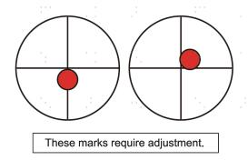
The laser mark should be near the centre of the hole. If the laser is not centred on the 1st mirror, cut the power to your laser and carefully adjust the laser tube in its brackets. This may require loosening the screws on its stand and adjusting its brace wheel. Be careful not to overloosen the screws and not to overtighten them. Only adjust one stand at a time.
