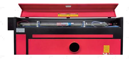
**Step 4.** Inside the main bay, remove the nylon cable ties from the X axis and the honeycomb table.
