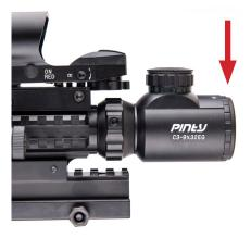
2. Adjust the reticle's brightness and color as needed using the illumination adjustment knob on the top of the eyepiece. Turning it towards you (clockwise) will first increase the brightness in the current color and then change to the next color, beginning at its lowest brightness. Turning it away (counterclockwise) will first decrease the brightness in the current color and then change to the next color, beginning at its highest brightness.
