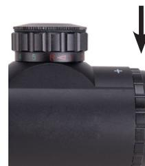
2. Adjust the reticle's brightness and color as needed using the illumination adjustment knob on the top of the eyepiece. Turning it towards you (clockwise) will first increase the brightness in the current color and then change to the next color, beginning at its lowest brightness. Turning it away (counterclockwise) will first decrease the brightness in the current color and then change to the next color, beginning at its highest brightness
